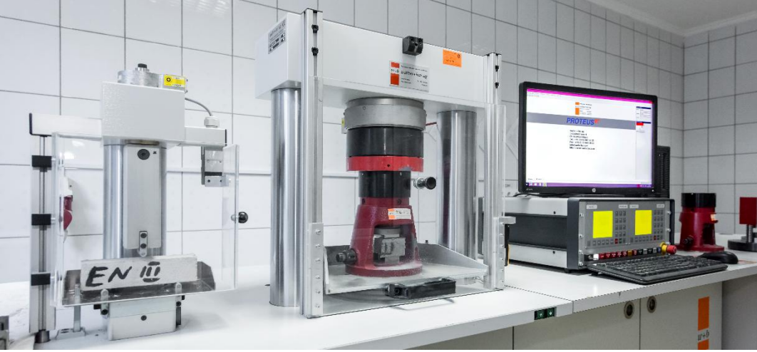
Fig. Testing machine Walter+Bai AG DB300/20 SUPER (PJSC "Ivano-Frankivskcement").
