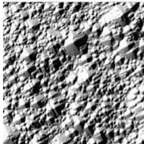
Random pyramids formed after alkaline texturing of monocrystalline silicon.
