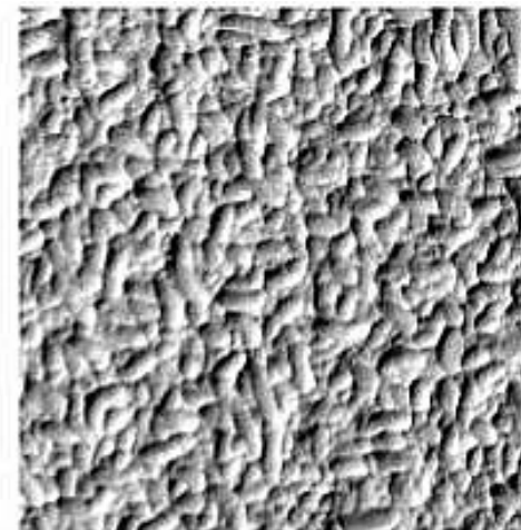
Worm-like structures formed after acidic texturing of multicrystalline silicon.
