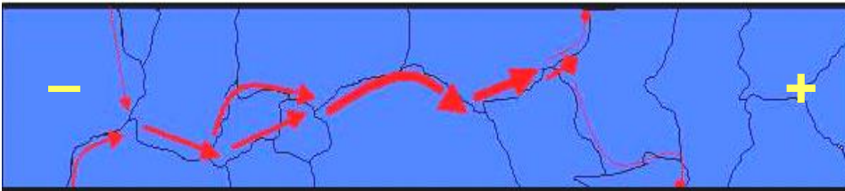
electromigration (local overheating)
